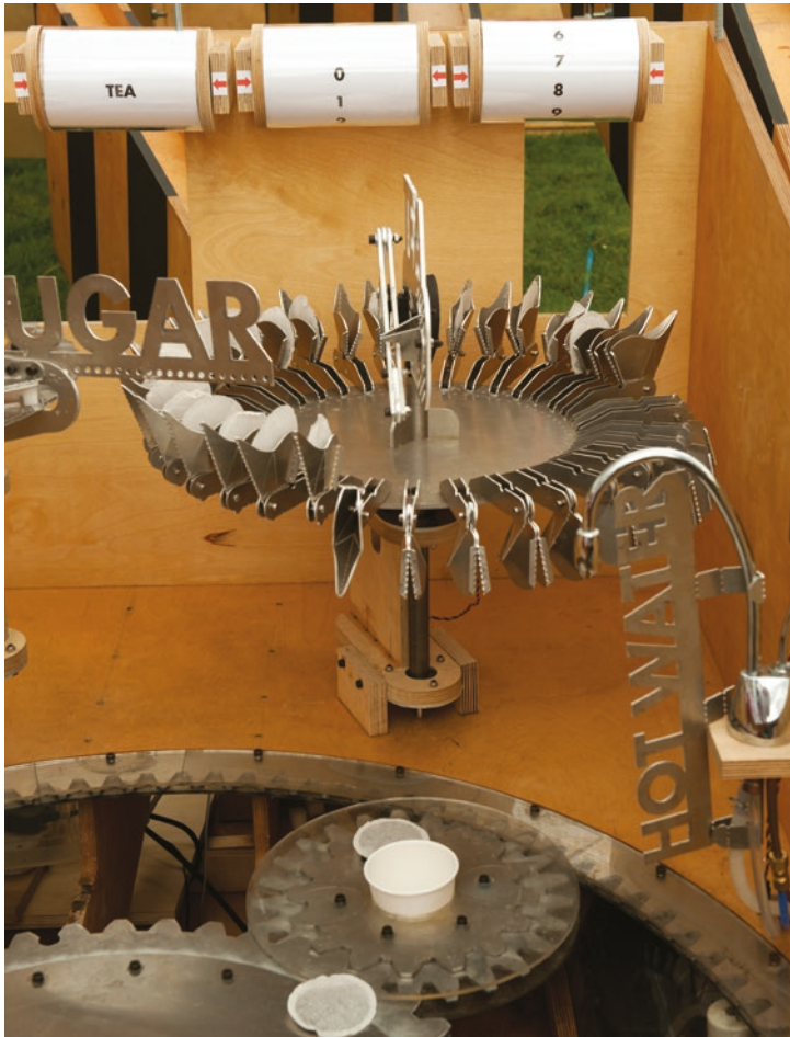
17 The teasmade showing cup delivery and the teabag dispenser
