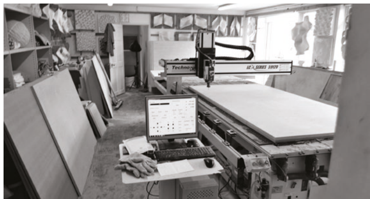
24 Panel prefabrication in the CNC workshop at Grymsdyke Farm
